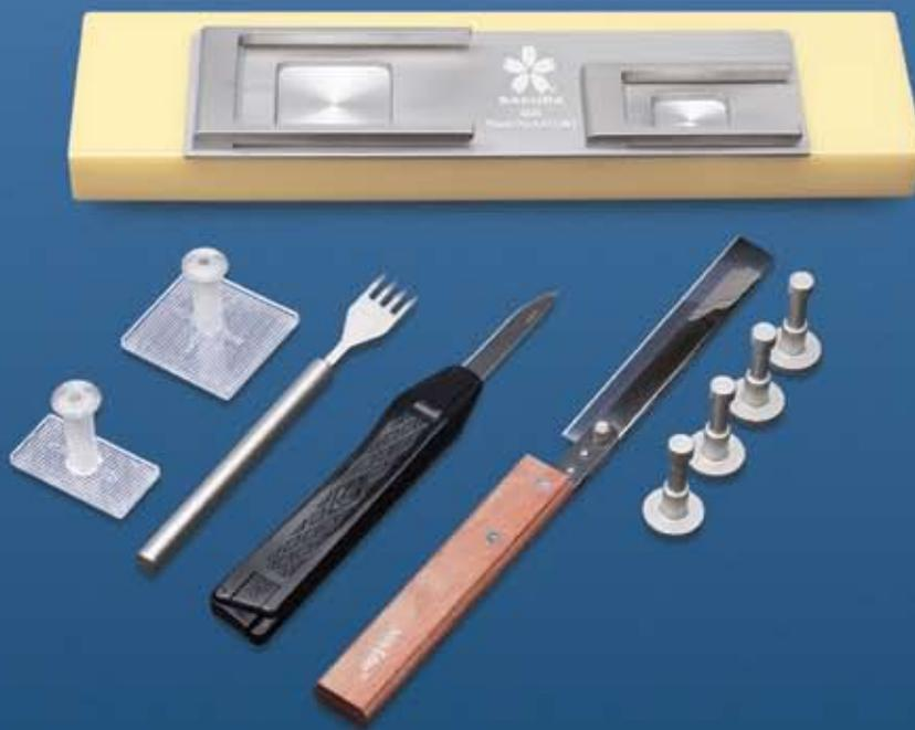
*The enhanced grossing wells allow for either left- or right-hand operation and can even be used on top of traditional grossing boards.*
