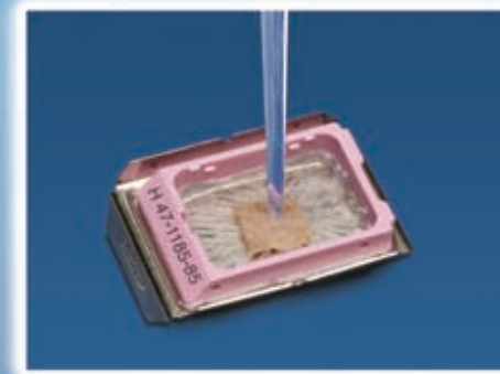
STEP 5—During paraffin dispensing, the specimen remains precisely oriented in the cassette.
