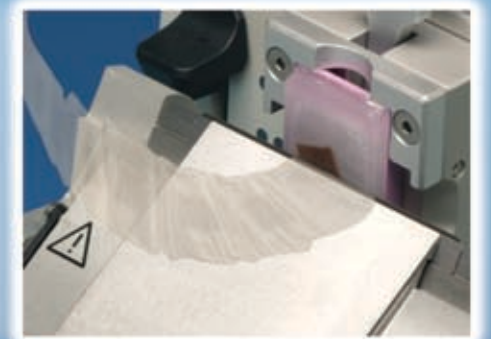
STEP 6—The Paraform® cassette design enables users to quickly obtain a paraffin ribbon.
